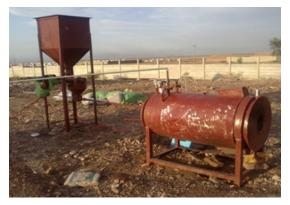
Figure 1: The cyclone combustor test rig.
