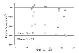
Figure 6: Effect of Air to Fuel Ratio on Furnace Temperature (Mesh Size 150 and 200).
